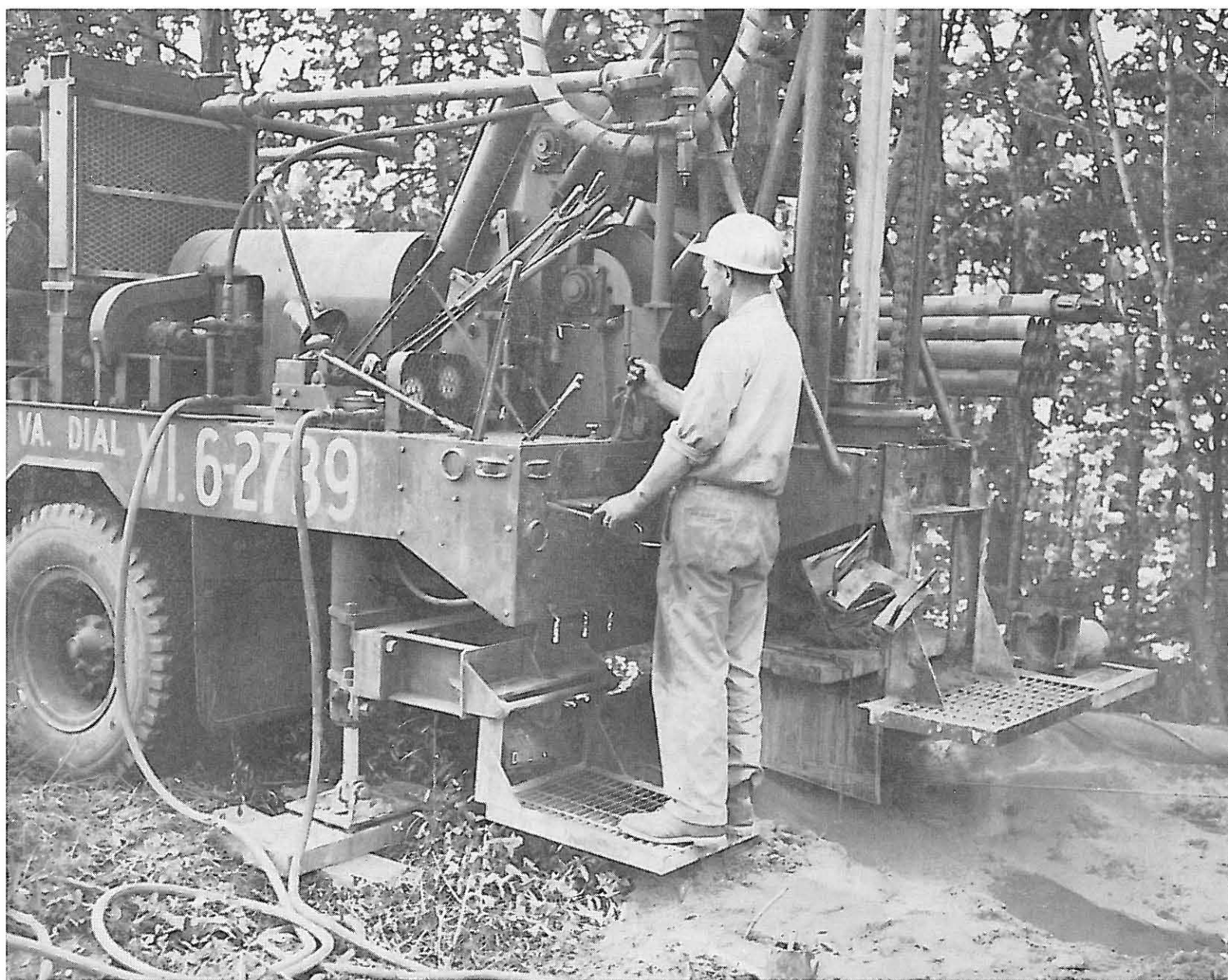
Close-up of simplified controls of Davey M-8A.
